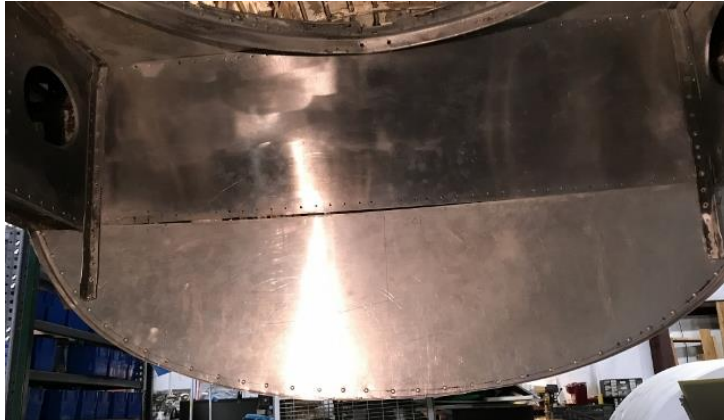
Back wall of the lower turret in place and almost ready for riveting
